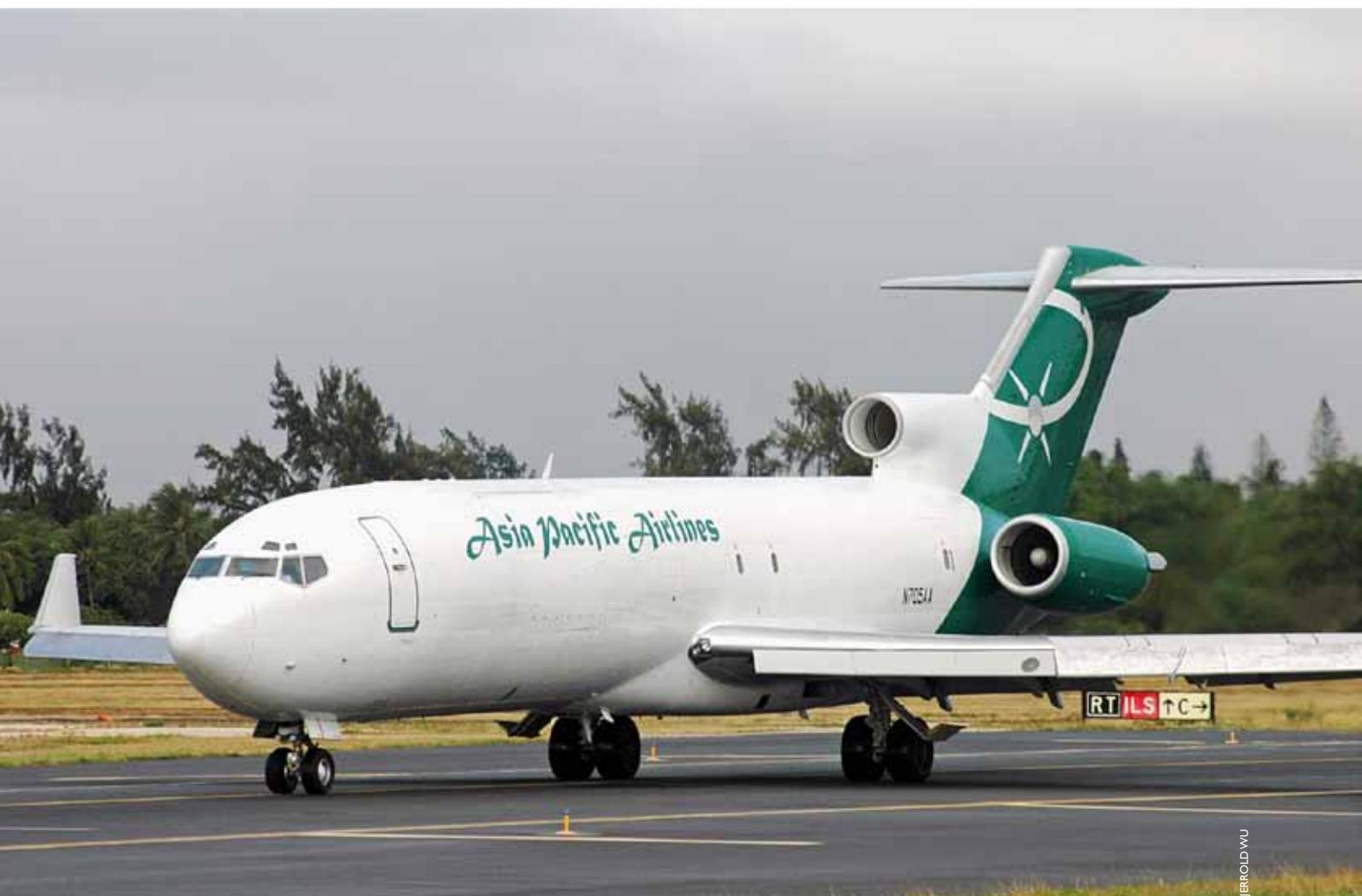
The Rohr/Goodrich Super 27 conversion of the 727 features Pratt & Whitney JT8D-217Cs in the outboard pods, with new hydraulic reversers, and the JT8D-17 (without reverser) retained in the center position. The changes result in reduced fuel burn, improved takeoff performance, and increased range and payload. This airplane was delivered new to American Airlines in 1978.
