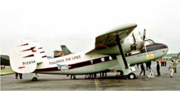
PAL briefly operated the eight-passenger Scottish Aviation Twin Pioneer (with Pratt & Whitney R-1340 engines instead of the original Alvis Leonides) on its Rural Air Service.
